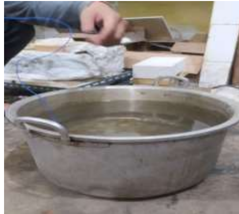
Gambar 3.6 Alat instalansi Quenching sistem media pendingin
