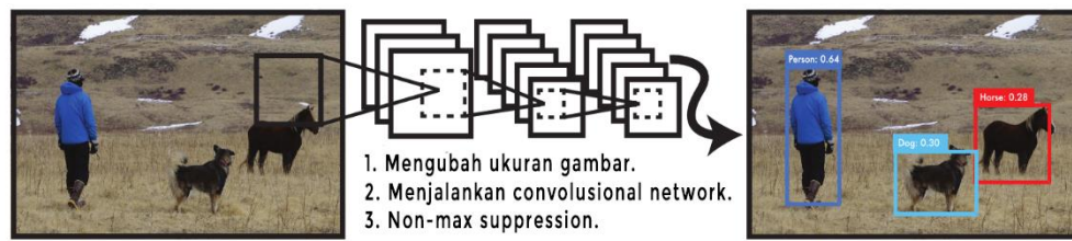
Gambar 9. Proses sistem deteksi YOLO (Redmon, et al., 2016).
