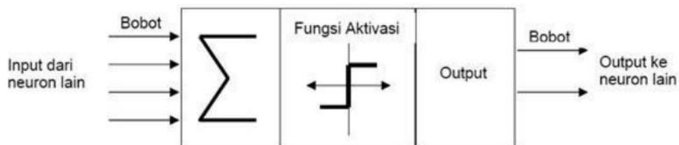
Gambar 3. Struktur *Neuron Artificial Neural Network*. (Sumber: Kusumadewi, 2003)
