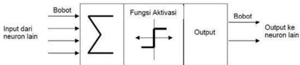
Gambar 3. Struktur *Neuron Artificial Neural Network*. (Sumber: Kusumadewi, 2003)
