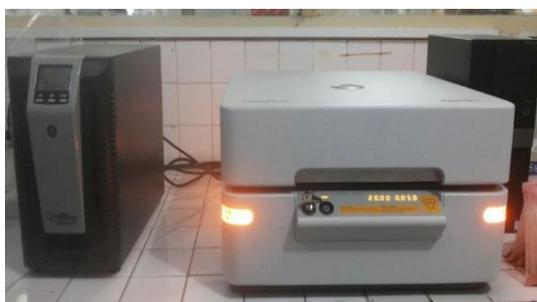
**Gambar 2.4** Alat XRF (PRTP - BRIN)
