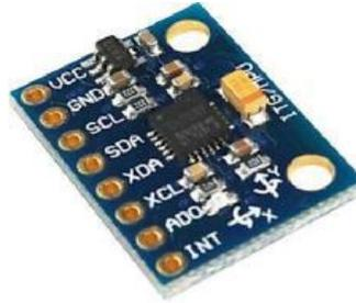
Gambar 2.4 Sensor MPU6050
