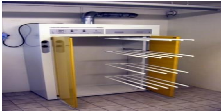
Gambar 4. Pengeringan Kabinet ( Cabinet Drying ).
