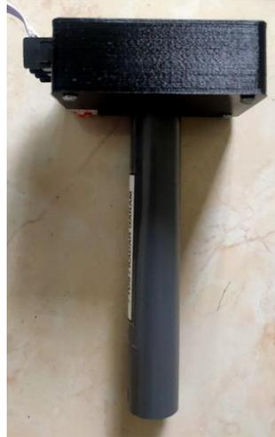
Gambar 2. 5. Sensor Salinitas
