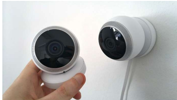
Gambar 17. Kamera CCTV ( Closed Circuit Televition ).
