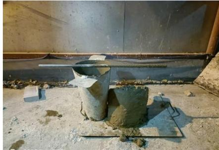
**Gambar 3.3** *Slump Test*
