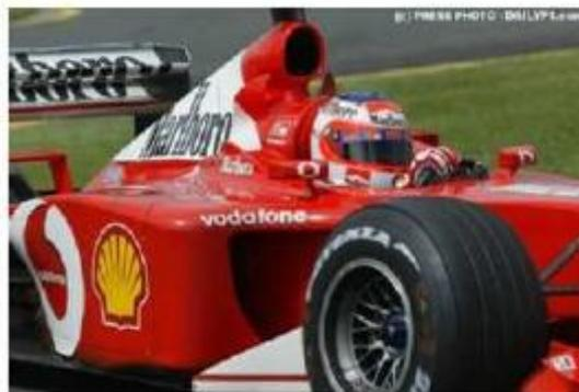
**Gambar 27.** *Scoop* Pada Mobil Balap. [Azizi, 2010]
