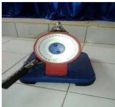
Gambar 8. Alat *Back and Leg Dynamometer*
