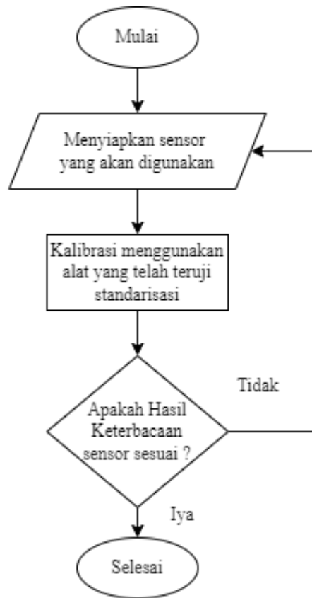
Gambar 3. 6 Diagram Alir Proses Kalibrasi Sensor
