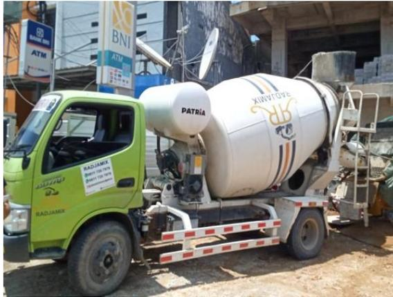
**Gambar 3.9.** Beton ready mix
