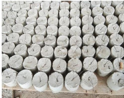
**Gambar 3.13.** Beton *decking*
