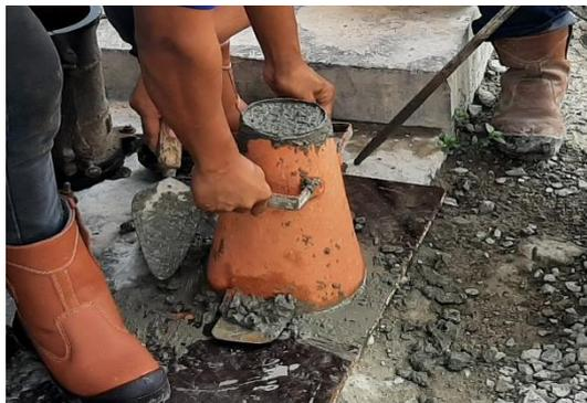
**Gambar 3.32.** Kerucut Abrams
