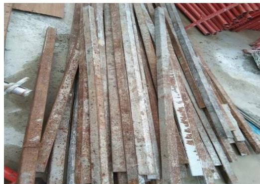
**Gambar 3.14.** Besi *Hollow* 50x50mm
