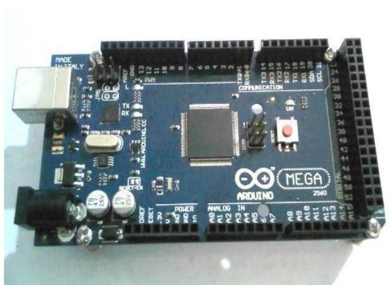
Gambar 3.8 Arduino Mega 2560
