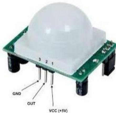
Gambar 2.4 Modul sensor PIR HC-SR501
