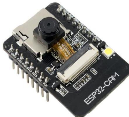
Gambar 2.7 ESP 32 CAM
