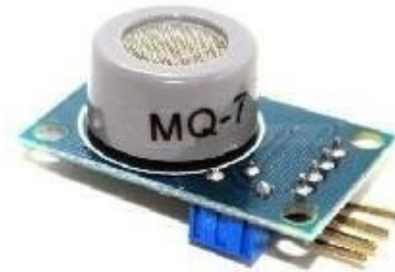
Gambar 2.1. Tampilan sensor MQ-7.
