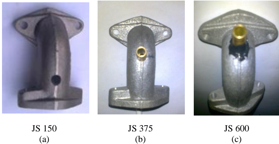
Gambar 39.a. Hasil pengeboran intake manifold JS 150
