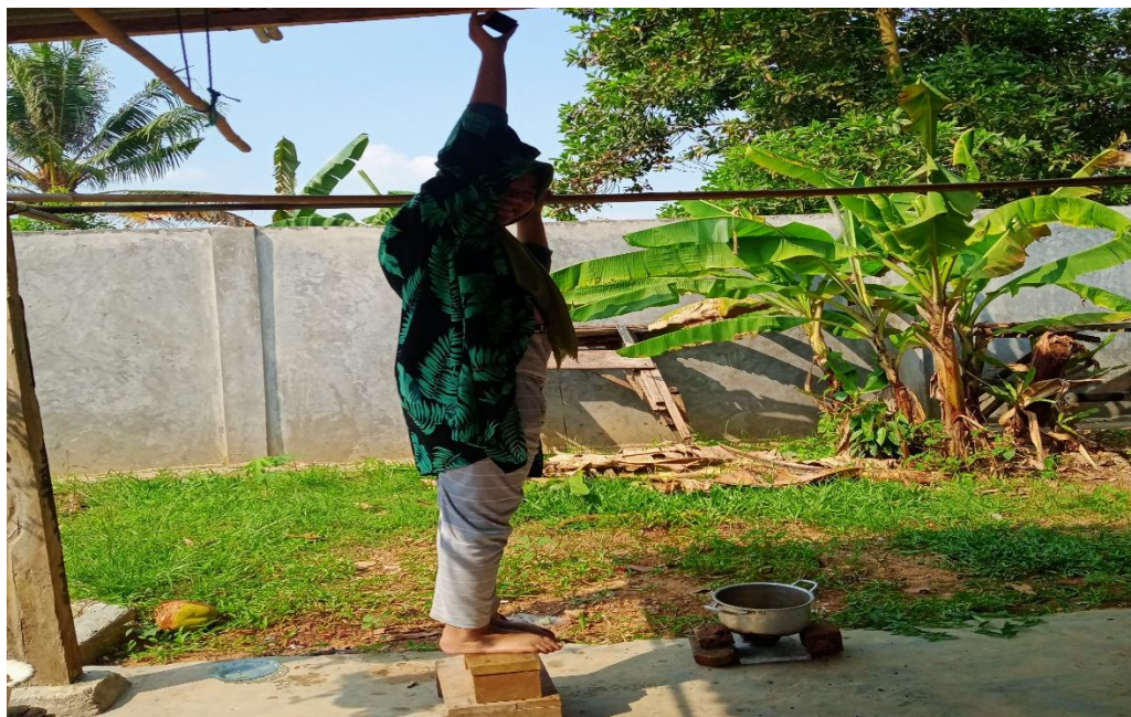
Gambar 13. Uji shatter resistance index biobriket.
