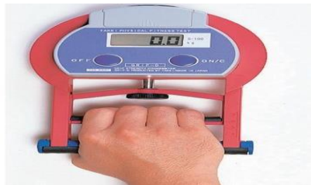
Gambar 3.3 Hand Grip Dynamometer Sumber gambar: Ismaryati (2008)
