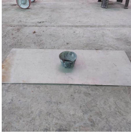
Gambar 3.11 Slum flow test.
