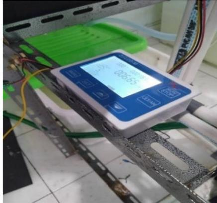
Gambar 3.5 *Water flow meter*
