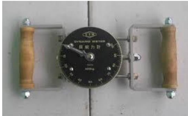
Gambar 12. Push and Pull Dynamometer (Ferdiansyah, 2017)
