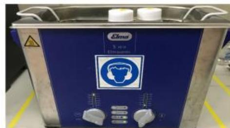
**Gambar 9. Ultrasonic Water Bath** (Aziz *et al.*, 2021)
