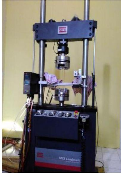
Gambar 38 Mesin MTS *Landmark* 100 kN
