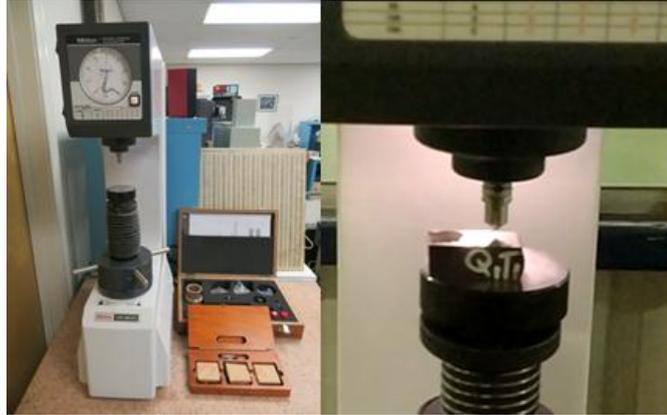
Gambar 36 Alat Uji Kekerasan Mitutoyo Hardness Tester model HR200
