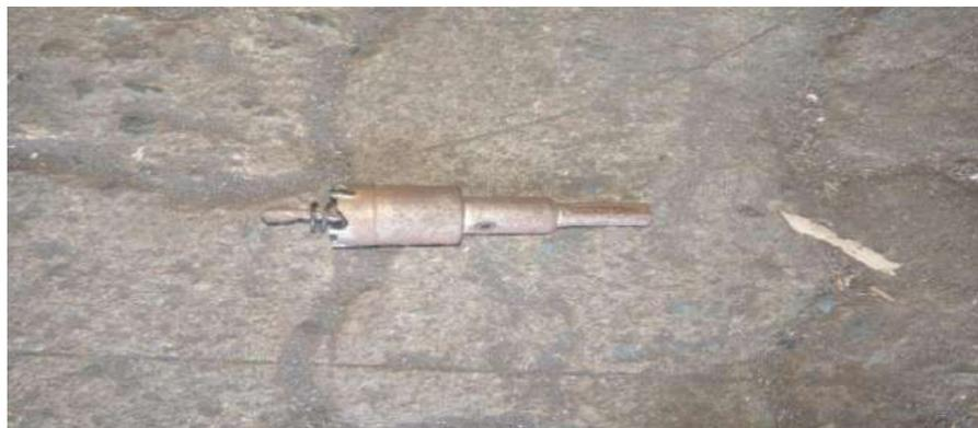
Gambar 3.15 *Hole saw* ukuran 25 mm
