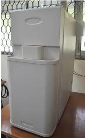
Gambar 3.3. Alat uji *ash fusion temperature*.
