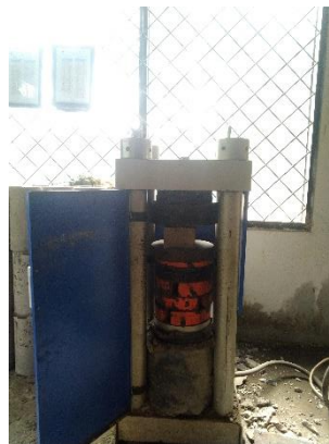
Gambar 9. Alat compression streng machine
