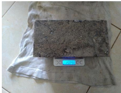
Gambar 11. Penimbangan paving block
