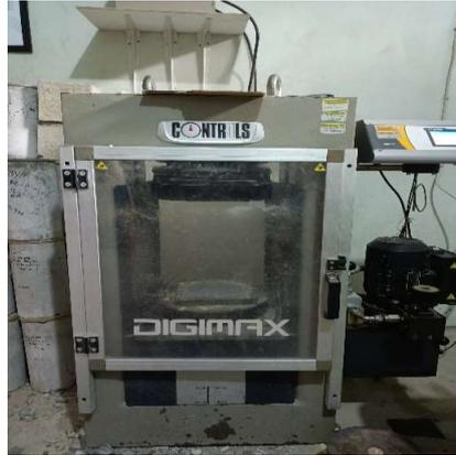
Gambar 10. *Digital Compression Testing Machine (CTM)*.
