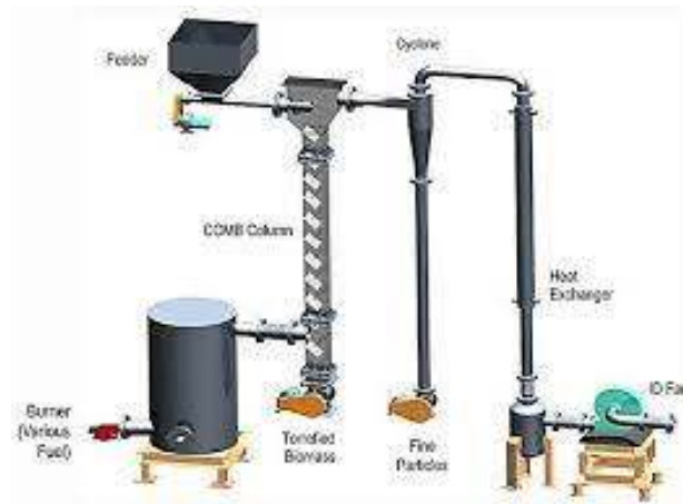
(Skema reaktor Counter-Flow Multi Baffle (COMB) (Sulistio dkk., 2020))
