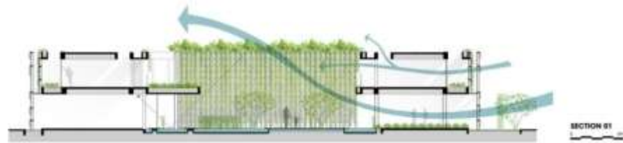
Gambar 2.6. Sistem cross ventilation Naman spa Sumber: www.archdaily.com
