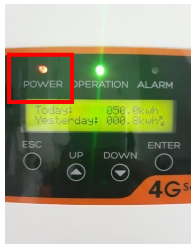
Gambar 3.11 LED Indicator “Power” ON
