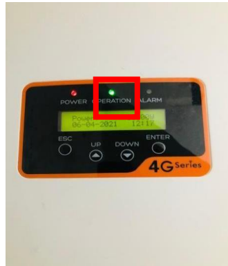
Gambar 3.12 LED Indicator “Operation” ON
