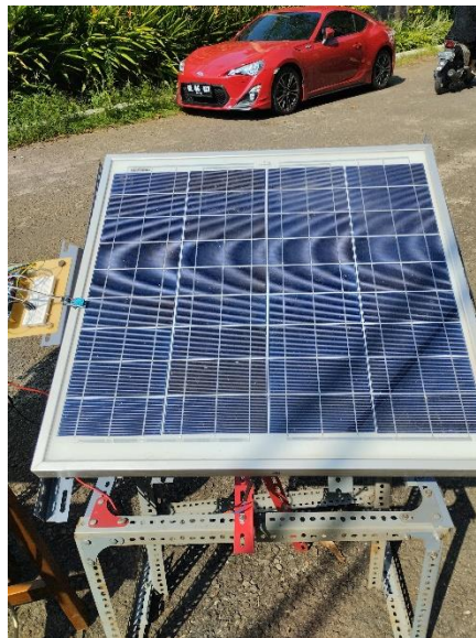
Gambar 3.9 Desain solar tracker panel surya tanpa reflector
