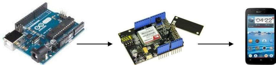
Gambar 3.7 Komunikasi SIM900 GSM *Shield*
