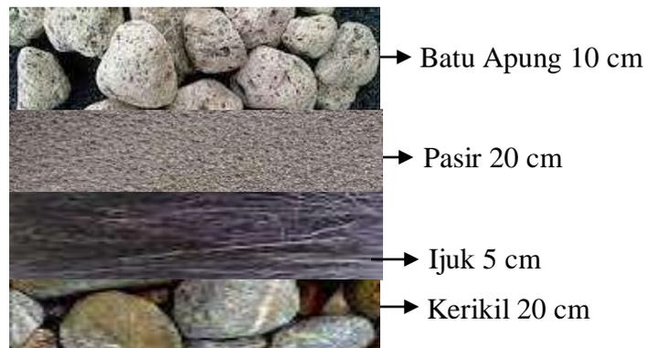
Gambar 13. Susunan filter mekanis
