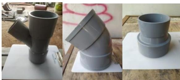
**Gambar 3. 35** Fitting Pipa PVC
