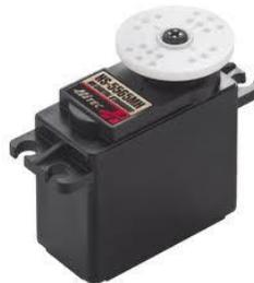
Gambar 25. Motor servo (DC) (Robotshop. 2013)
