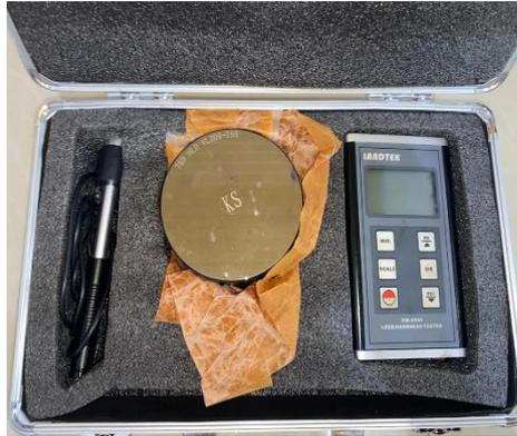
Gambar 12. *Hardness tester*
