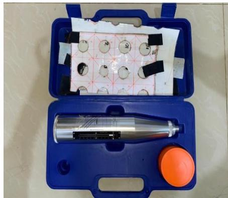
Gambar 13. *Hammer test*
