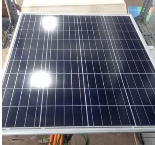
Gambar 2.3. Panel surya *polycrystalline*
