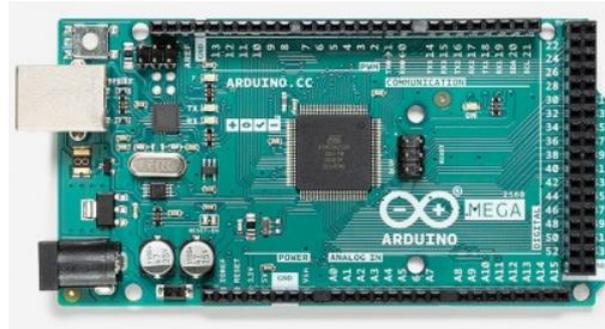
Gambar 5. Arduino Mega 2560
