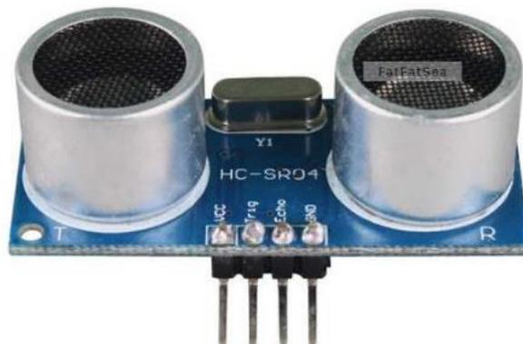
Gambar 9. Sensor Ultrasonik
