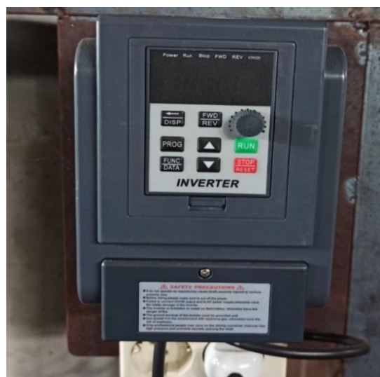
Gambar 3.6 Inverter AC motor single phase
