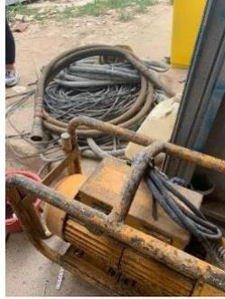
**Gambar 3.5.** *Concrete Vibrator*
