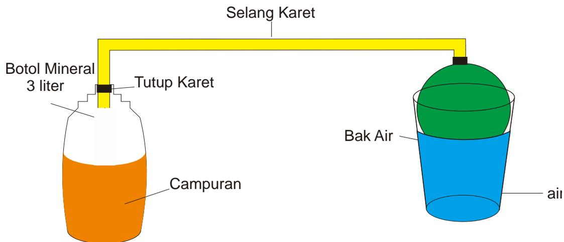
Gambar 2. Skema Biogas Sistem Batch
