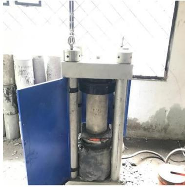
Gambar 3.18. CTM (*compression testing machine*).
