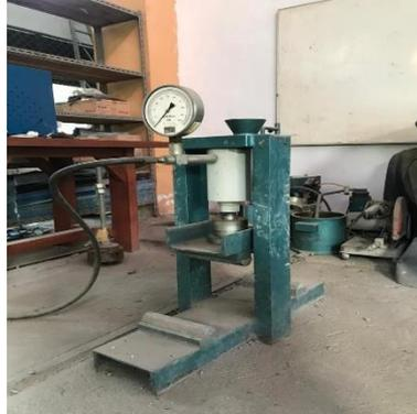
Gambar 3.22. *Flexural testing frames*.
