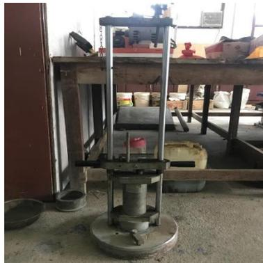
Gambar 3.23. ITM (*impact testing machine*).
