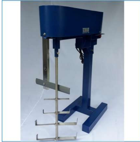
Gambar 2. 1 Mesin mixer sabun
