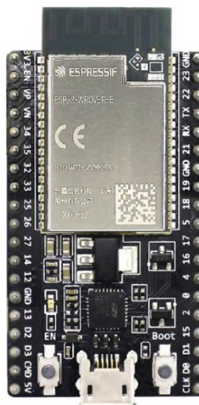
Gambar 2. 3 Modul ESP32 DevKitC
