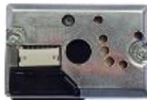
Gambar 2.4 Sensor Debu GP2Y1010AU0F
