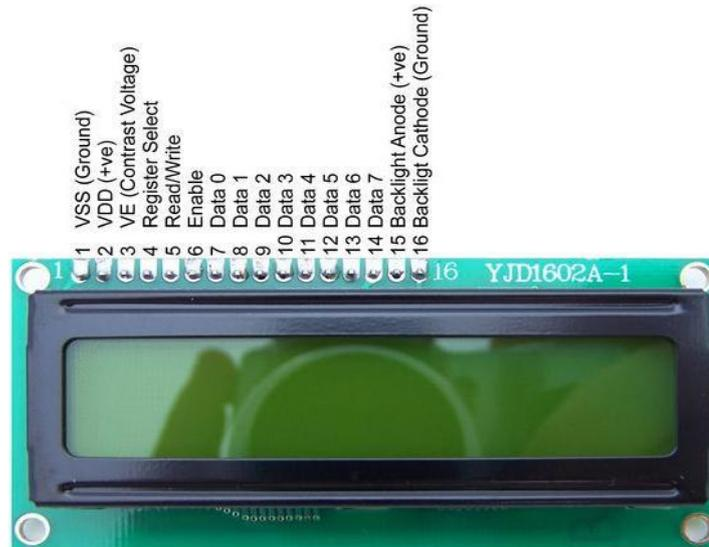
**Gambar 2.8** LCD 16x2
