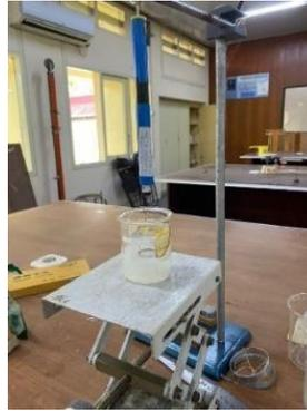
**Gambar 3.2** Alat tensiometer.
