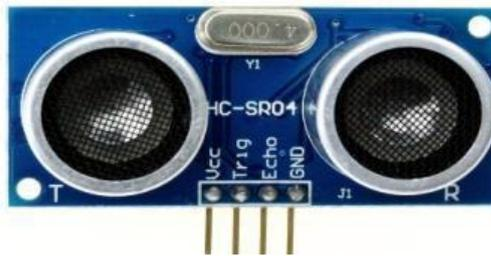
**Gambar 2.8 Sensor Ultrasonik HC-SR04**
