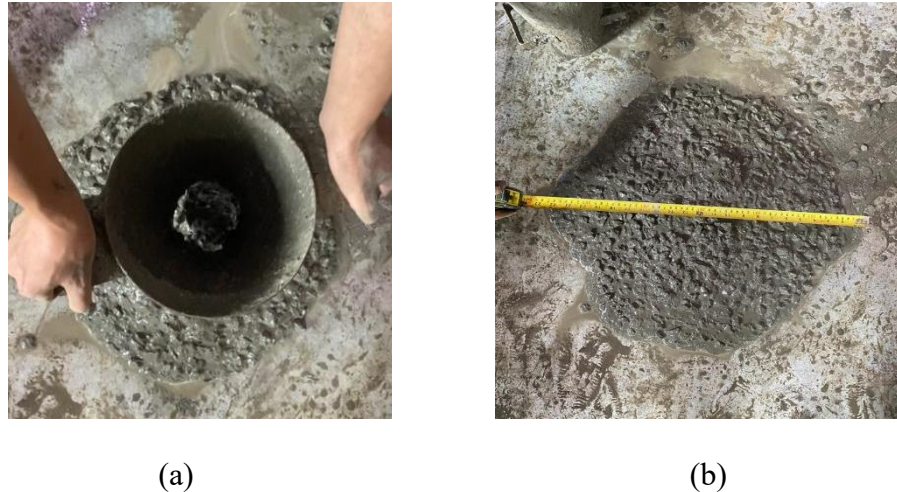
Gambar 3.2. Slump Flow Test (a), pengukuran diameter (b).
